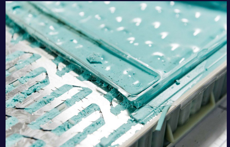
Image of adhesives used in a Tesla Model 3 battery pack Image taken from TeslaOwnersOnline.com
